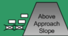
3-Bar VASIS for Wide Body Aircraft (Ignore Downwind Bars)
